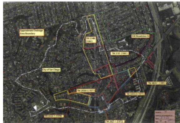
Water in the tributary area drains into curb inlets, underground pipes (some publicly and some privately owned), through the Ruiz pipe, and ultimately discharges near a freeway. The image below shows part of the system’s flow near the Property.
